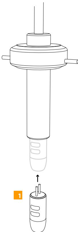
**3** Once the fitter is inside of the top opening, rotate until the holding posts allow the lamp to sit center of the glass.
