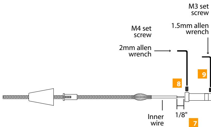
**10** While inserting the inner wire into the connector look through the set screw hole to make sure that the stripped portion of the inner wire contacts end of the connector.
