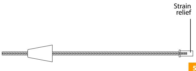
**6** Slide the outer wrapped wire back to expose the inner wire.
