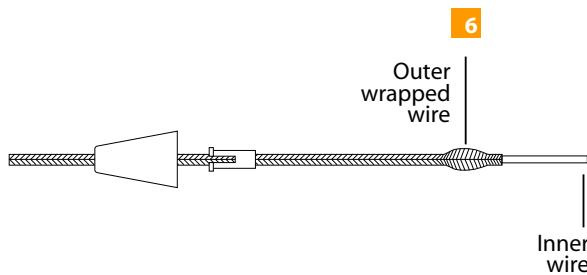
**7** Strip 1/8" from end of the inner wire. Make sure that the stripped portion is not greater than 3/16".
